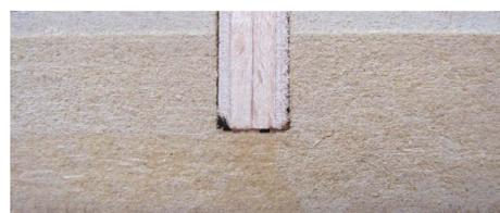
Shelves were freely supported and loaded for 28 days with distributed static load related to 100 kg/m<sup>2</sup> which correspond to L 50 according to DIN 68874. The elastic deflection was measured immediately after the load was applied and hourly for the first 8 hours and after that the readings were taken daily. Additionally by using FEM software program SAP 2000 the deflection were evaluated theoretically for six different constructions of shelves.
