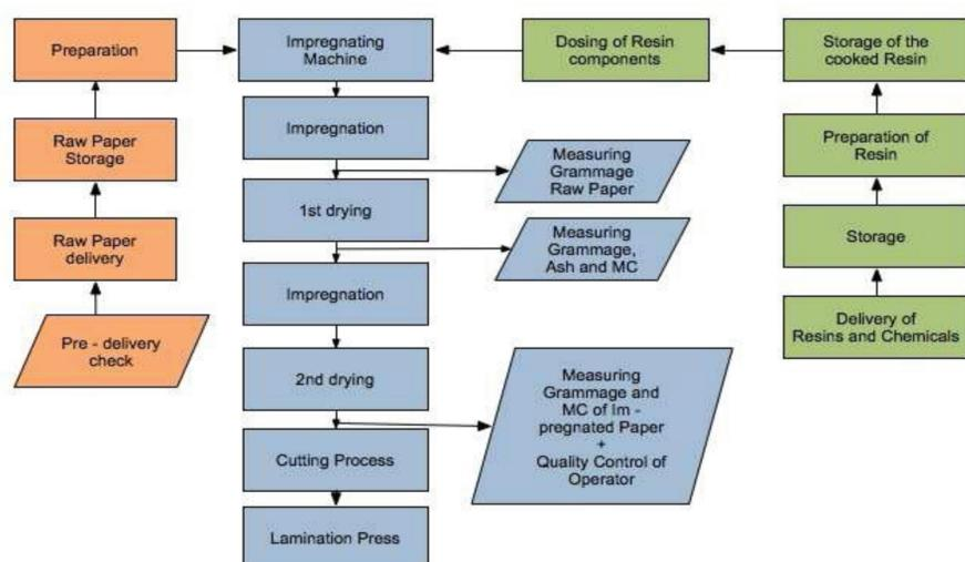
Figure 1: Process chart of Impregnated paper production
